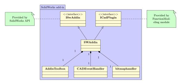
Figure B.3: UML-diagram of SolidWorks add-in
