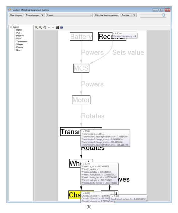
Figure 7.12: While dragging the time slider, the simulation results are shown in tooltips and the components are visible depending on the value of their visibility variable. The difference between not filtering the results (a) and filtering the results (b) is clearly visible. The difference between invisible (b) and visible (c) components is also shown
