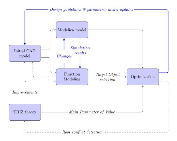
Figure 5.1: Overall workflow (figure 1.1 repeated). The thick blue arrows show the interactions that are worked on during this project. The dashed black arrows stand for interactions that are not implemented yet and that are not worked on during this project. Available interactions are shown using normal black arrows.
