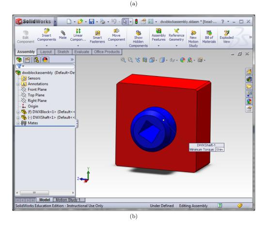
Figure 6.2: In the overview of design guidelines (a), the user can select the ones that are visible in SolidWorks (b). The *callout* in this example shows that the motor shaft should at least be able to provide a torque of 5Nm
