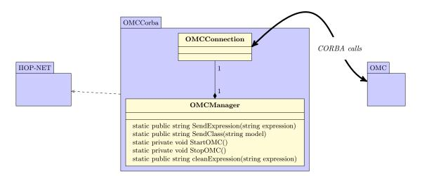
Figure B.2: UML-diagram of OMCCorba module
