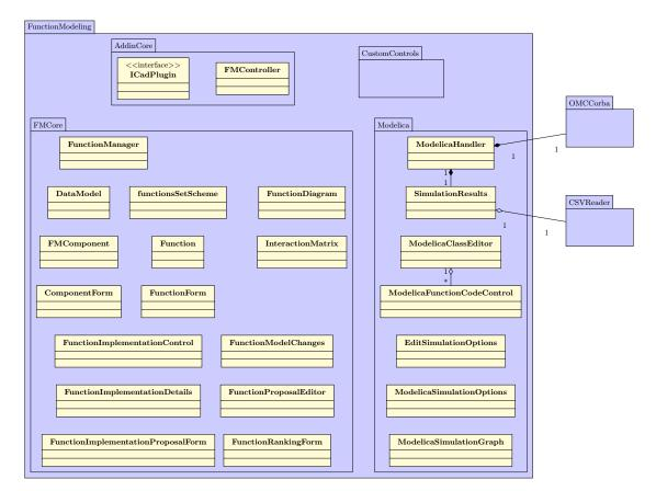
Figure B.1: UML-diagram of FunctionModeling module
