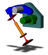
Figure A.1: Valve-cam assembly from the SolidWorks 2011 Motion Studies tutorial
