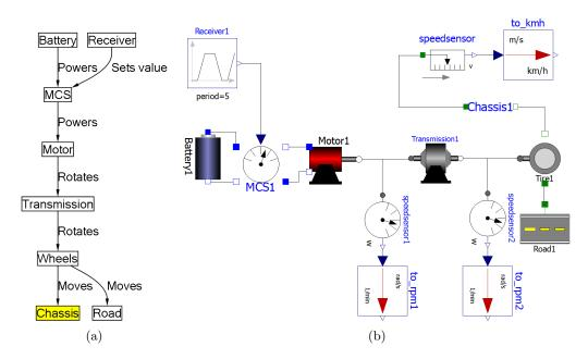
Figure 7.8: Function model diagram (a) of the RC-car and corresponding Modelica model (b)
