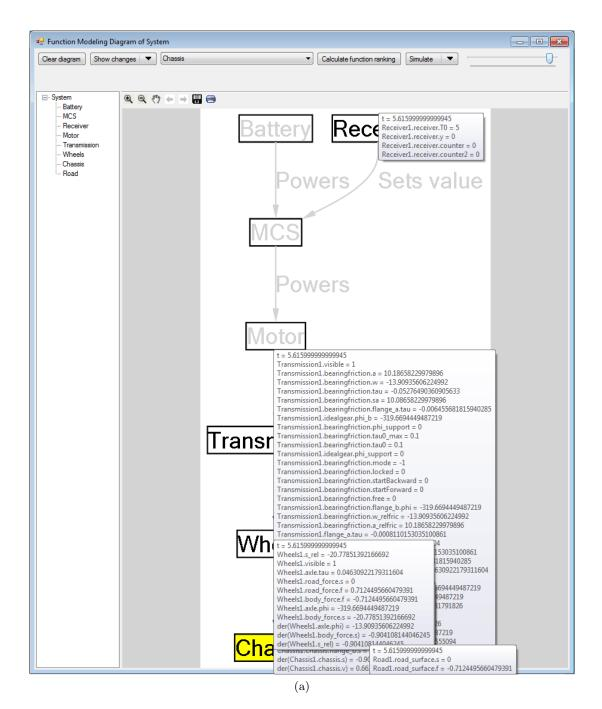
Figure 7.12: While dragging the time slider, the simulation results are shown in tooltips and the components are visible depending on the value of their visibility variable. The difference between not filtering the results (a) and filtering the results (b) is clearly visible. The difference between invisible (b) and visible (c) components is also shown
